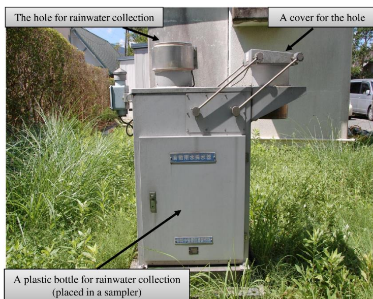
Fig. 2.2. A picture showing an auto atmospheric wet-dry sampler (US-750, Ogasawara Keiki Seisakusho).
